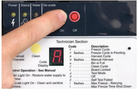
Note: Main Controller Lights and Switches are Duplicated on the Lower Light and Switch Panel
