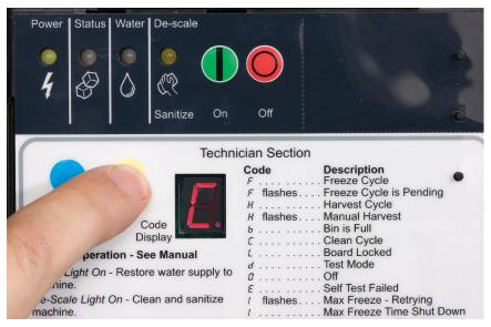
After 6 months of power up time, the De-Scale & Sanitize light will be switched On. It will switch off after the machine has been run through the cleaning process.
