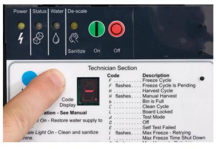
Put the control into the standby mode, then push and Hold the Clean button for 3 seconds. A "-" will be displayed. The pump and purge valve will be On for 30 seconds, repeat as needed to drain the reservoir.
