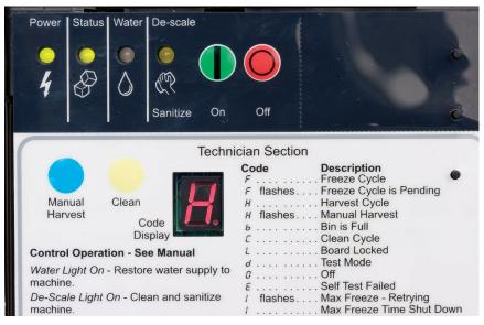
The harvest cycle starts when the ice thickness sensor is contacted by water running over the ice. During harvest, the display indicates an *H*.
